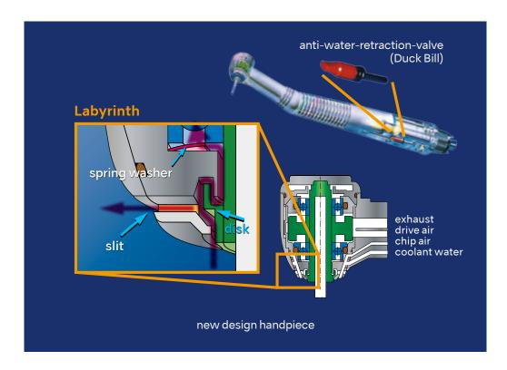
[Fig. 3] Handpieces tested left: new type handpiece with the Labyrinth right: conventional handpiece
