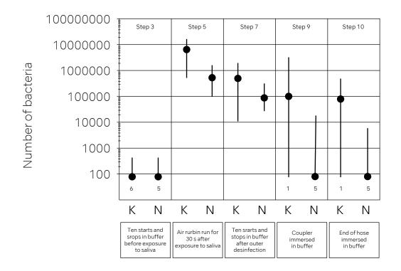
[Table 1.] The number of bacteria detected in various steps in testing Kavo (K) and NSK (N) handpieces according to fig. 1. The bacteria were cultured on blood agar for 2 d in an atmosphere of air with 5% carbon dioxide. <100 means that no bacteria were detected on the blood agar plates.</p>
